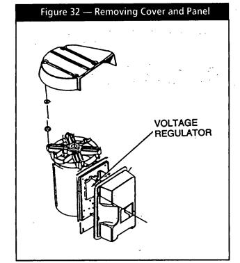
With frequency at 62 Hertz, AC voltage should read 124 volts. If voltage is incorrect, slowly turn the VOLT-AGE ADJUST POT on voltage regulator (Figure 33) until AC voltage is correct.
